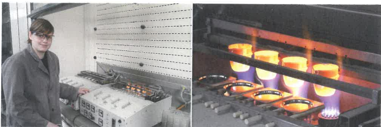
Figure 1: Fused tablets are produced from the clinker and cement samples for the X-ray fluorescence analysis.
