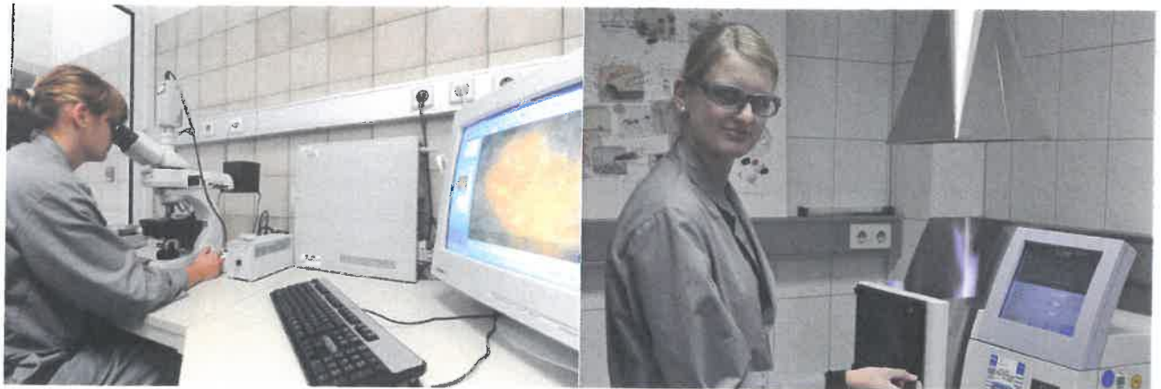
Figure 2: In addition to the standard physical and mechanical measurements (compressive and bending tensile strength), polarisation microscopy and atomic absorption spectrometry (AAS) are also used in the central laboratory to deal with specific problems.
