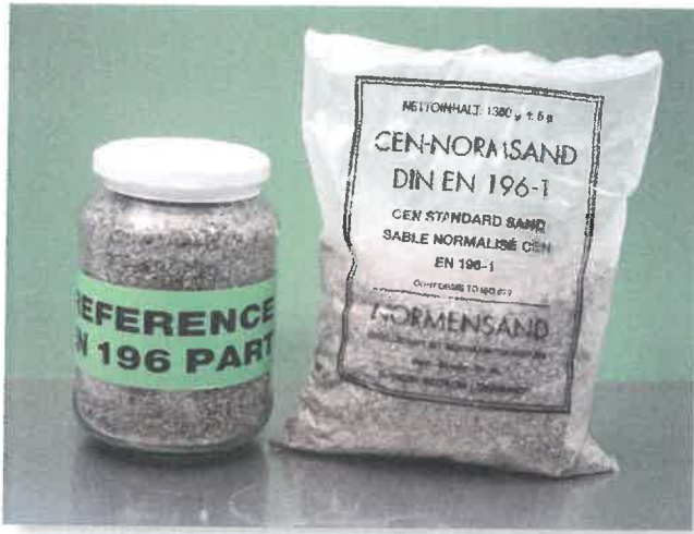
Figure 1: In accordance with EN 196-1, CEN standard sand must be packed in pouches containing 1350 \pm 5 g. Three mortar prisms can be produced with one pouch. Specifying the pouch weight minimizes weighing errors in the laboratory. The CEN reference sand, i.e. the fundamental standard for the CEN test sand, is stored and sold in glass jars packed by Normensand GmbH.
