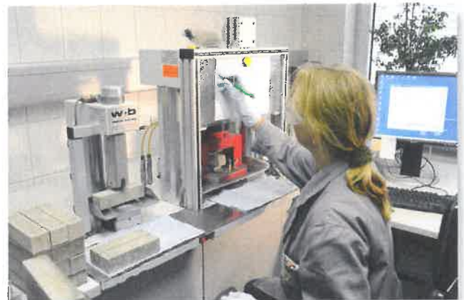
Figures 2–4: HeidelbergCement AG's central laboratory in Ennigerloh has been optimized for high product throughput. The standard mortars are stored in special steel basins. The results of the mortar compressive strengths are automatically assigned to the sample recorded in the LIMS and evaluated statistically.
